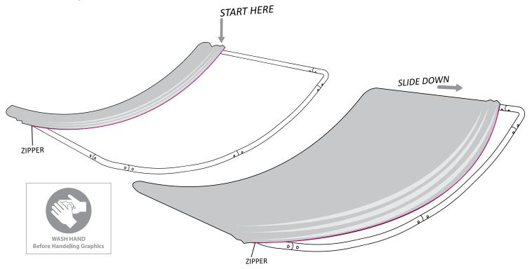
**STEP 4.** When the zipper reaches the bottom the fabric becomes tighter. Pull the fabric firmly with one hand around the bottom tube while zipping the bottom closed with the other hand.
