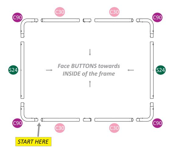
**STEP 2.** Start in this corner. Push the button with your thumb while sliding the tubes together. Twist as needed to click the button into the hole.
