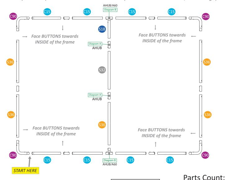
**STEP 2.** Start in this corner. Push the button with your thumb while sliding the tubes together. Twist as needed to click the button into the hole.
